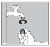
2. Set the hose correctly by loosening the ring nut. After positioning the inlet hose, be sure to tighten the ring nut again to prevent leaks.
